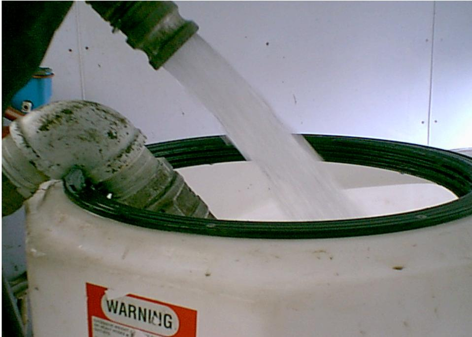
Clean, recycled water for reuse in the Oil Water Separator
